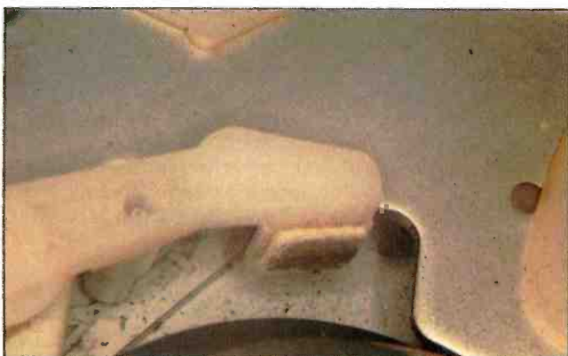
Figure 4. Dirt on the sub-brake T pressure pad.
